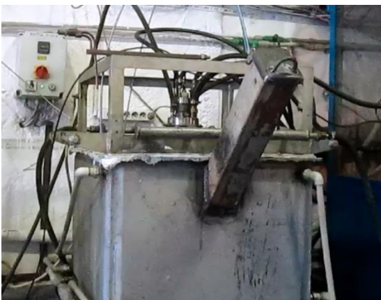
Fig. 3. Chamber furnace of 30 kg/h of SCW productivity with plasma torch of 90 kW
