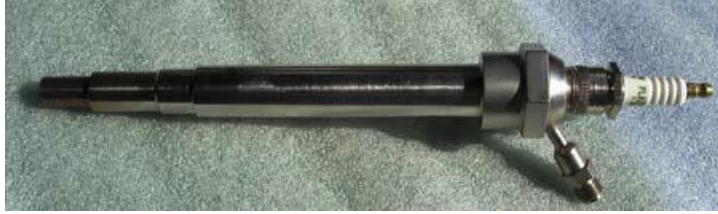
Fig. 2. Supersonic Plasma Igniter
