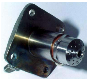
Fig. 5. Appearance of a plasma fuel nozzle for gaseous fuel on the left and for liquid fuel on the right
