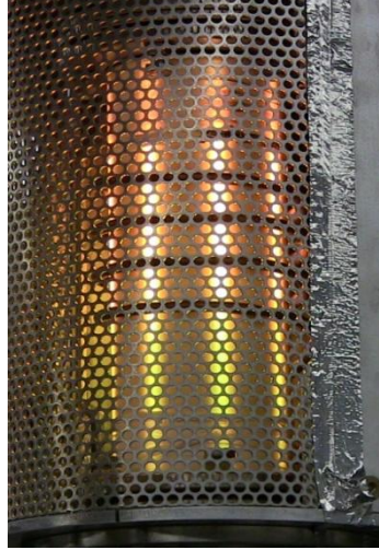
Fig. 6. The effect of unmixed argon (top) and nitrogen (bottom) plasma layers existence in the RF torch with reverse vortex flow
