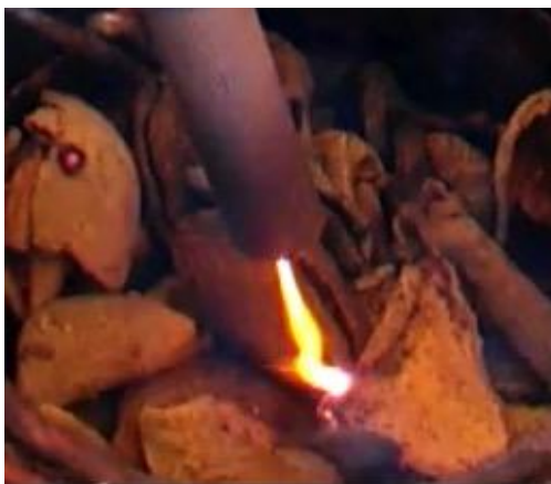
Fig. 2. Dielectric breakdown operation with almond hulls.
