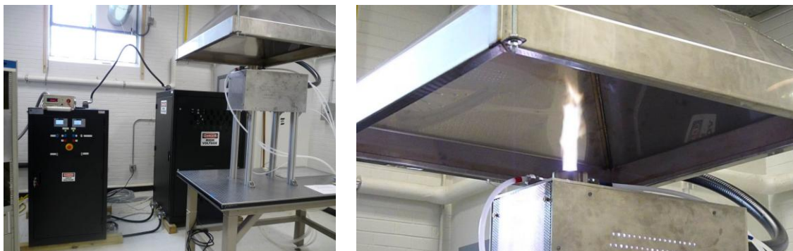
Fig. 9. Two-modular APT-100 (left) and its metal-ceramic torch in operation on air
